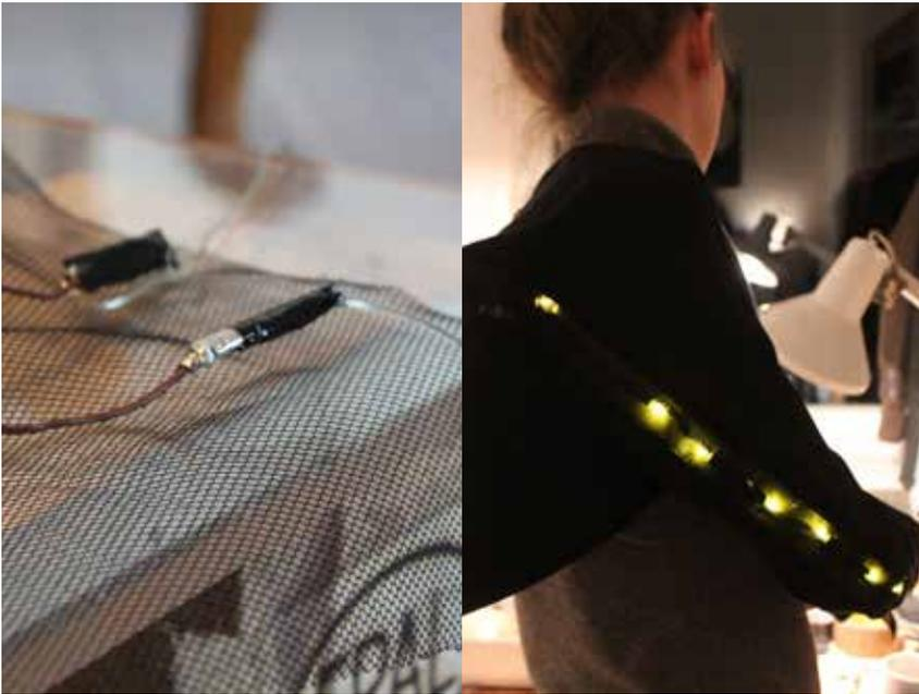
To make the back brace, we sewed three components into the suit. The light source is covered with thin layers of a mosquito net style fabric that dims and diffuses the light.
